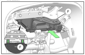
8. Secure stock power supply module (F) with new screw (3) and retained nut (E). Torque fastener to specification.
