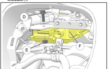
3. Remove and retain power supply module (f) from RH fairing bracket and set aside.
