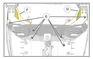
7. Reinstall lower backrest piece ① with three retained screws ①. Torque screws to specification.
