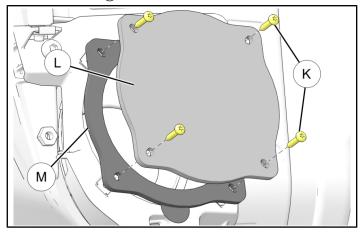
b. Connect electrical connectors to new speakers ① and set in place. Secure speakers using retained screws (6). Torque fasteners to specification.
