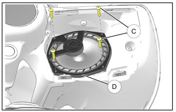
3. Lift out speaker D and unplug electrical connector E. Discard speaker.
