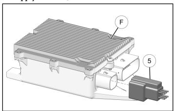
7. Install retained stock power supply module (F) into LH fairing bracket opening. Ensure two tabs slide into bracket as shown. Plug connector into module.
