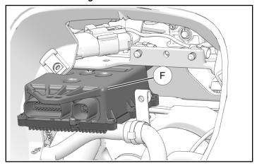
4. Install new power control module ② into RH fairing bracket in place of removed module. Ensure two tabs slide into bracket as shown. Plug in two connectors into module.
