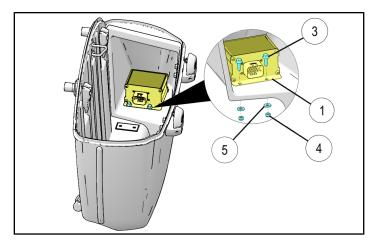
3. Locate the amplifier cover plate ②. The cover plate will be mounted to hide the rear portion of the saddlebag, as shown in the figure. Clean the mounting surfaces on the saddlebag with isopropyl alcohol or similar to ensure proper adhesion. Remove the backing paper from the two Velcro straps and install the amplifier cover plate ② to the LH saddlebag. Apply pressure to the top and bottom of the plate to ensure proper adhesion before separating the Velcro strips.
